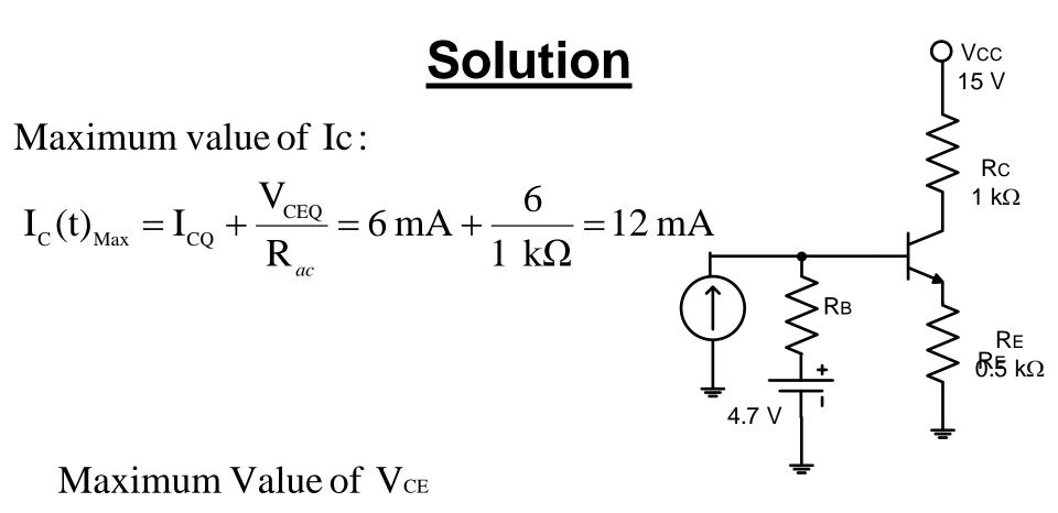
$V_{CE}(t)_{Max} = I_{CQ}R_{ac} + V_{CEQ} = 6 \text{ mA.1 } \text{ k}\Omega + 6 = 12 \text{ V}$
