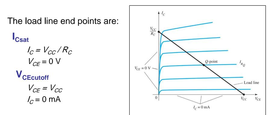
The *Q*-point is the operating point where the value of  $R_B$  sets the value of  $I_B$  that controls the values of  $V_{CE}$  and  $I_C$ .
