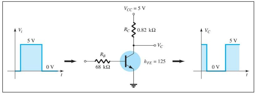
For Vi = 0V  $I_B = 0$   $I_C = 0$   $V_{CE} = V_{CC}$  $\therefore$  BJT is in Cut - off Mode & Vc =  $V_{CE(cut0ff)} = V_{CC} = 5V$
