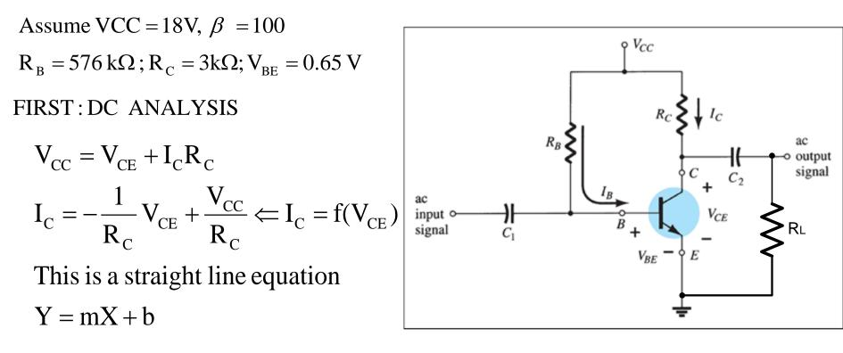
$$I_{B} = \frac{V_{CC} - V_{BE}}{R_{B}} = \frac{18 - 0.65}{576 \text{ k}\Omega} = 30 \text{ }\mu\text{A}$$
