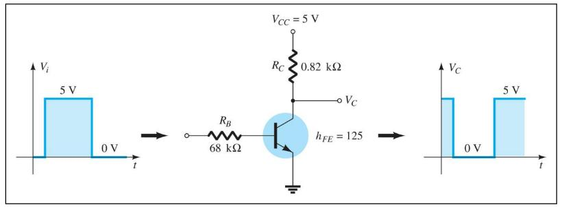
$$I_{C(sat)} = \frac{5}{0.82 \text{ k}\Omega} = 6.1 \text{ mA}$$
