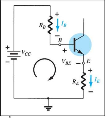
Also, in order to guarantee operation in linear mode we choose  $0.1 V_{CC} \le V_E < 0.2 V_{CC}$
