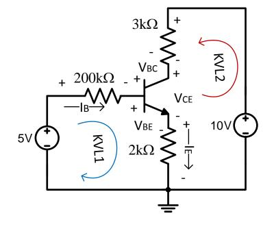
∴ Q1 is in active mode and the assumption is true we can also verify that the BC junction is reverse biassed which is required so that the BJT operates in active mode
