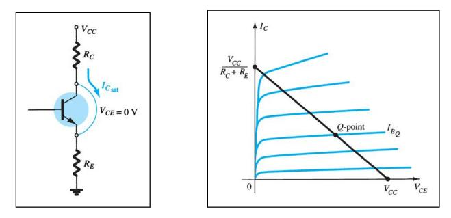
The endpoints can be determined from the load line.
