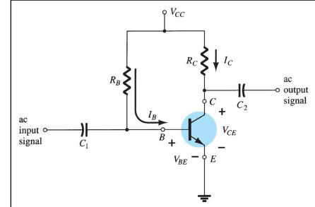
$\label{eq:stable} \begin{array}{l} \mbox{for} \\ 50 \leq \beta \leq 150 \\ 10.56 \ \mu A \geq \ I_B \geq 9.489 \ \mu A \\ 0.528 \ m A \leq \ I_C \leq 1.423 \ m A \\ 6.89 \ V \geq \ V_{CE} \geq 3.31 \ V \\ \hdots \frac{I_{C(max)}}{I_{C(min)}} = \frac{1.423 \ m A}{0.528 \ m A} \cong 2.7 \end{array} \begin{array}{l} \mbox{Improved,} \\ \mbox{but not} \\ \mbox{very} \\ \mbox{stable} \end{array}$
